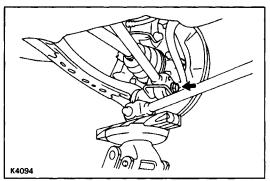
(c) Torque the No.1 suspension arm bolt of the axle carrier side.
