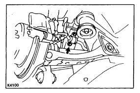
**3. REMOVE STABILIZER BRACKET WITH BUSHING** Remove the four bolts and stabilizer bracket with bushings.
