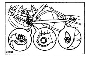
(b) Temporarily install the suspension arm No.2 with a bolt, toe adjust cam and toe adjust plate.HINT: Face the mark to the rearward.
