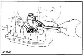
(d) Remove the two bolts and pull out the park/neutral position switch from manual valve shaft.
