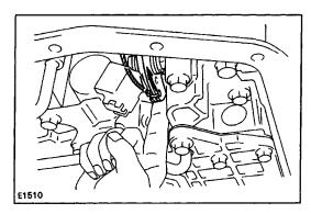
(c) Connect the throttle cable to the cam.
