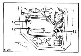
(b) Install the oil strainer with the three bolts.
