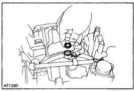
12. REMOVE SECOND BRAKE APPLY GASKET
