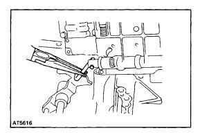
(c) While disconnecting the manual valve connecting rod from the manual valve lever, remove the valve body.
