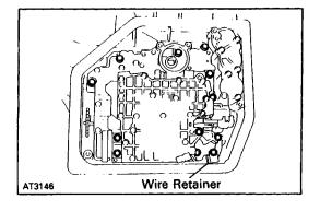
(b) Remove the twelve bolts and wire retainer.
