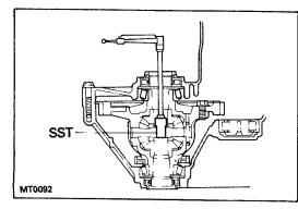
HINT: Align the matchmarks on the differential case and contact the ring gear.
