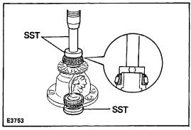
(b) Using SST and a press, install the side bearing. SST 09550–10012 (09252–10010, 09556–10010, 09560–10010)
