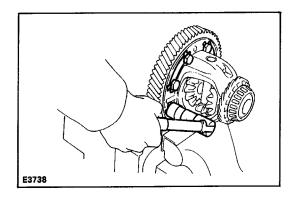
(c) Remove the eight bolts and four lock plates.
