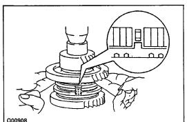
(d) Install the needle roller bearing, 1st gear and synchronizer ring.
