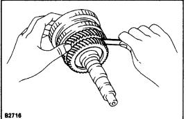
**7. INSPECT SECOND GEAR THRUST CLEARANCE** Using a feeler gauge, measure the 2nd gear thrust
