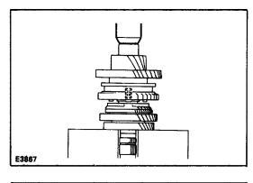
(e) Using a press, install the 3rd driven gear.
