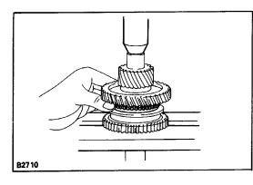
(f) Using a press, install the 1st gear and No. 1 hub sleeve.
