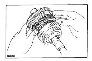
SST SST MT0063 5. REMOVE THIRD DRIVEN GEAR, SECOND GEAR, NEEDLE ROLLER BEARING, SYNCHRONIZER RING AND SPACER
