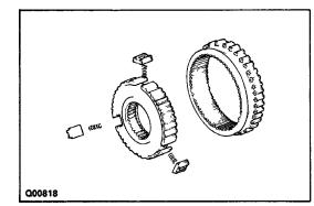
8. REMOVE NO. 1 HUB SLEEVE, SHIFTING KEYS AND SPRINGS FROM NO. 1 CLUTCH HUB
