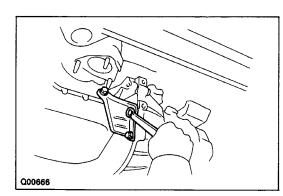
2. INSTALL STIFFENER PLATE Torque: 37 N-m (380 kgf-cm, 27 ft-lbf)
