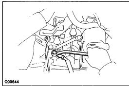
16. INSTALL EACH CABLE Torque: 21 N-m (210 kgf-cm, 15 ft-lbf)
