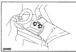
4. CONNECT ENGINE LEFT MOUNTING Torque: 63 N-m (650 kgf-cm, 47 ft-lbf)
