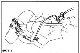
**18. INSTALL CLUTCH RELEASE CYLINDER** Install the release cylinder and tube with the four bolts.
