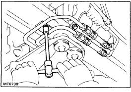
**4. INSTALL TUBE SET BOLTS** Install the two bolts.
