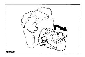
(d) While holding transfer output slightly, pull out whole transaxle.
