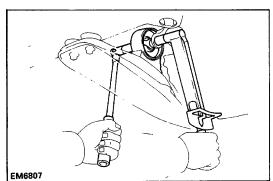
**(**b) Tighten the front through bolt.
