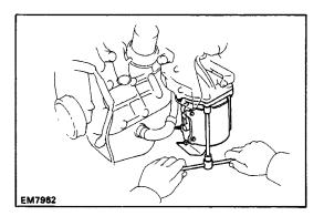
(c) Remove the three bolts, two nuts, catalytic converter, cushion, retainer and gasket.
