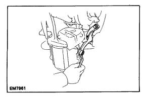
(d) Install the LH converter stay with the three bolts.
