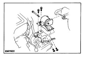
(b) Remove the through bolt, four bolts and LH mounting insulator.
