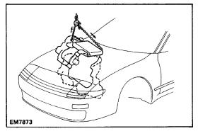
(e) Lift the engine out of the vehicle slowly and care—fully.
