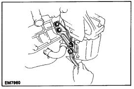
(c) Install the RH converter stay with the four bolts.
