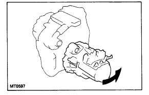
(c) Move the transmission case cover to the arrow in the illustration.
