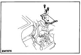
(c) Remove the three bolts and LH mounting bracket.
