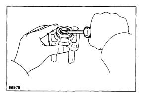
6. IF NECESSARY, REPLACE CONTROL SHAFT COVER OIL SEAL
