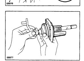
5. REMOVE CONTROL SHAFT COVER AND DUST BOOT
