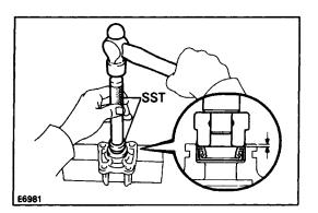
(b) Using SST and a hammer, drive in a new oil seal. SST 09620-30010 (09627-30010, 09631-00020)
