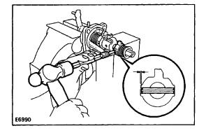
(c) Using a pin punch and hammer, drive in the slotted spring pin.
