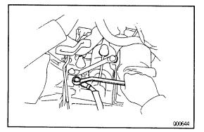
16. INSTALL EARTH CABLE Torque: 21 N-m (210 kgf-cm, 15 ft-lbf)
