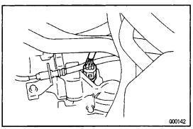
10. DISCONNECT VEHICLE SPEED SENSOR CONNEC-TOR
