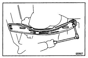
3. INSTALL CENTER CROSSMEMBER Install the center crossmember with the four bolts. Torque: 52 N-m (530 kgf-cm, 38 ft-lbf)
