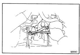
**17. INSTALL ENGINE MOUNTING LEFT STAY** Install the mounting left stay with the bolt and nut. **Torque: 21 N–m (210 kgf–cm, 15 ft–lbf)**
