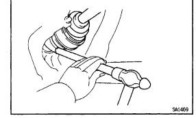
Oil:. Gear oil super (08885–02106) or equivalent Recommended oil Oil grade: API GL-3, GL-4 or GL-5 Viscosity: SAE 75W-90 Above  $-18^{\circ}$  C (0°F) SAE 90 Below –18°C (0° F) SAE 75W Capacity: 2.6 Liters (2.7 US qts, 2.3 Imp.pts) **10. INSTALL UNDER COVERS** 11. INSTALL FRONT WHEEL AND LOWER VEHICLE Torque: 103 N-m (1,050 kgf-cm, 76 ft-lbf) 12. INSTALL ENGINE LEFT MOUNTING BOLTS OF ENGINE LEFT MOUNTING UPPER SIDE Torque: 63 N-m (650 kgf-cm, 47 ft-lbf)
