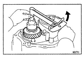
(b) Install and torque the new lock nut. **Torque: 123 N-m (1,250 kgf-cm, 90 ft-lbf)** HINT: The lock nut has LH threads.
