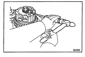
(c) Using a screwdriver and hammer, tap in the snap ring.
