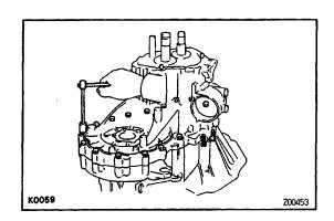
(c) Install and torque the seventeen bolts.
