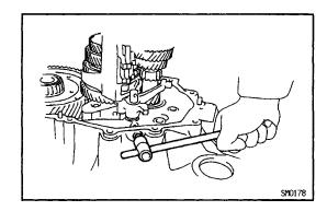
(c) Apply sealant to the plug threads.
