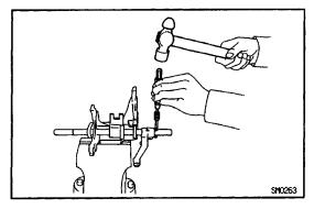
(g) Using a pin punch and hammer, drive in the slotted spring pin to the No. 1 fork shaft.
