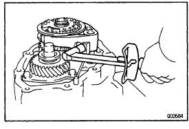
(b) Install and torque the set bolt.
