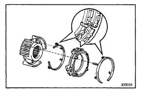
(c) Install the No.5 synchronizer rings with key springs to the No.3 clutch hub.
