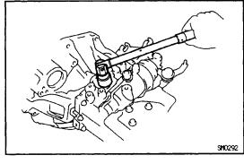
28. INSTALL BACK-UP LIGHT SWITCH Torque: 44 N-m (450 kgf-cm, 33 ft-lbf)
