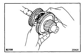
(c) Place the synchronizer ring on the gear and align the ring slots with the shifting keys.
