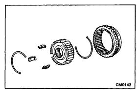
6. REMOVE NO.1 HUB SLEEVE, SHIFTING KEYS AND SPRINGS FROM NO.1 CLUTCH HUB
