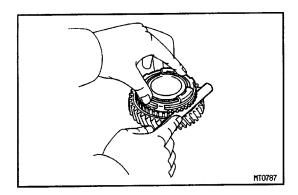
(c) Measure the clearance between the synchronizer ring back and gear spline end.
