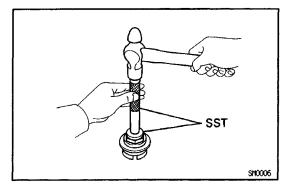
(b) Using SST and a hammer, tap in a new oil seal until its surface is flush with the shaft cover surface.
