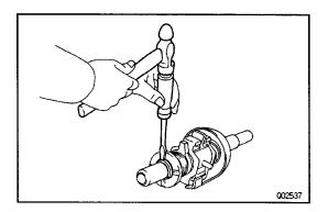
(b) Using a screwdriver and hammer, tap in the E-ring.
