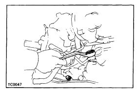
(e) Tighten the union bolt holding the oil pipe to the cylinder block.
