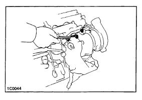
(c) Tighten the four nuts holding the turbocharger to the exhaust manifold.
