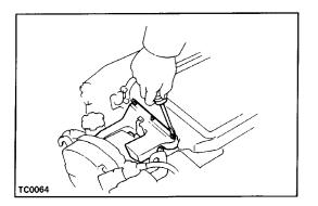
**13. REMOVE CHARGE AIR COOLER COOL AIR INLET** Using a clip remover, remove the seven clips and air inlet.
