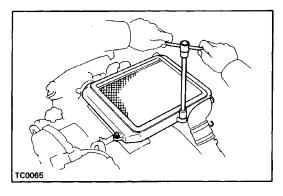
**12. INSTALL CHARGE AIR COOLER PROTECTOR** Install the protector with the three bolts.
