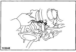
(d) Tighten the two nuts holding the oil pipe to the turbocharger.
