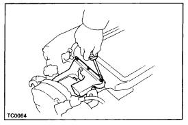
**13. INSTALL CHARGE AIR COOLER COOL AIR INLET** Install the cool air inlet with the seven clips.
