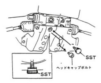
With the rack centred and the sensor correctly adjusted the steering rods should be of equal length and the wheels at the correct alignment.
